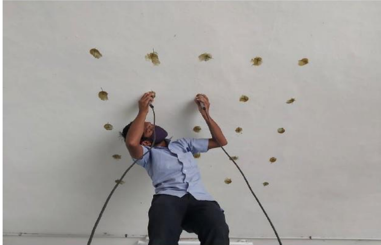
Photo 13 A view of the UPV test in progress in the RC Slab of the ground floor by indirect method of measurement
