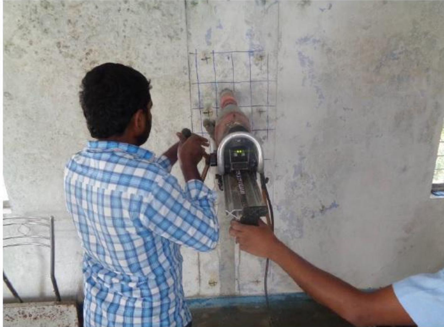
Photo 14 A view of the core drilling test in progress in a RC Column of the First Floor
